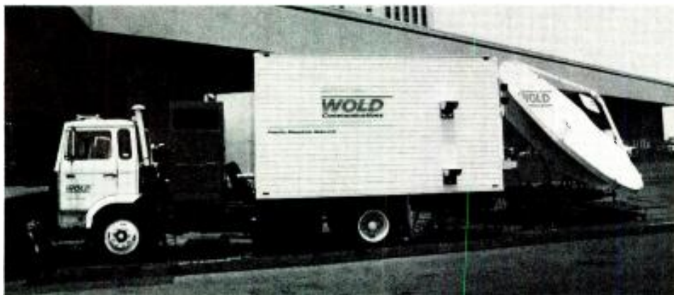
Wold transportable antenna and truck, with diesel powered generator, prepares for transmission.
