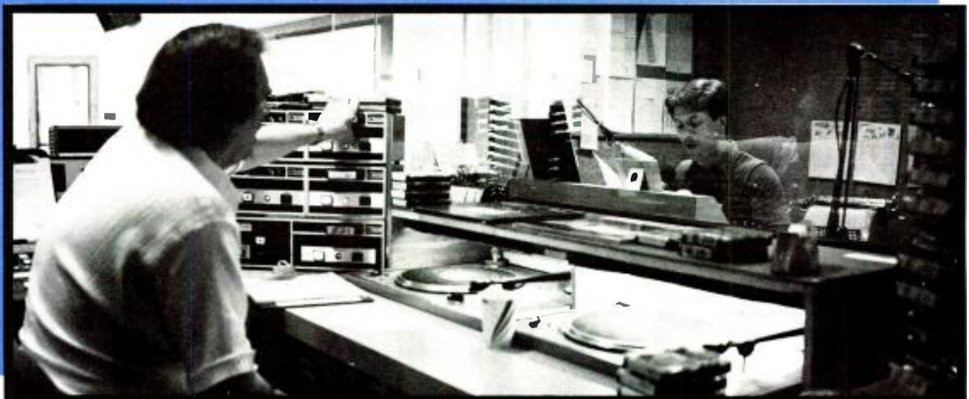
Operator, from his seat, easily starts cart machines or turntables or operates console (close on left).
