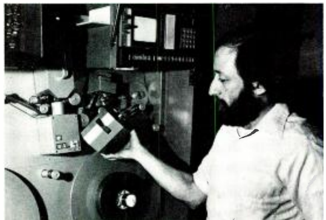
An engineer checks the scanner assembly for the Bosch CCD telecine. Film—16 or 35 mm, positive or negative—is moved continuously past the solid state elements.
