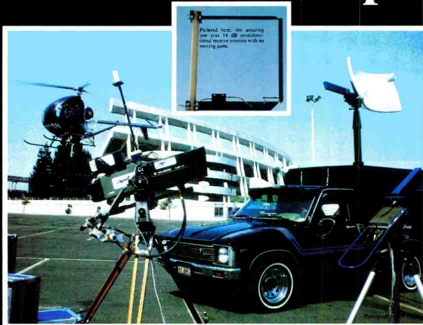
Pictured here: Hughes 300 and BMS microwave, camera mounted omni and transmitter, portable yagi antenna. Truck mounted 2x4 di
