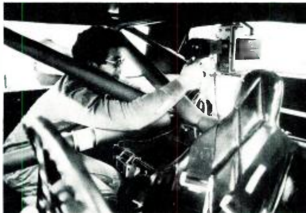
ABC Engineering Labs' Harvey Waldman adjusts focus servo on Panasonic AK-710 POV camera.
