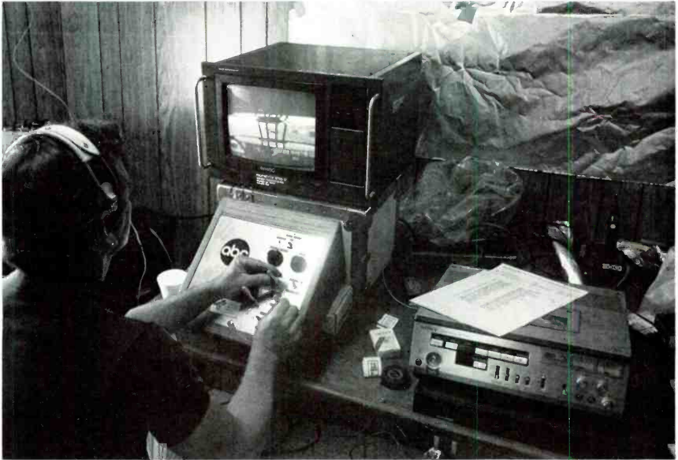
Camera operator controls remote pan/tilt head and various camera controls from specially designed panel.
